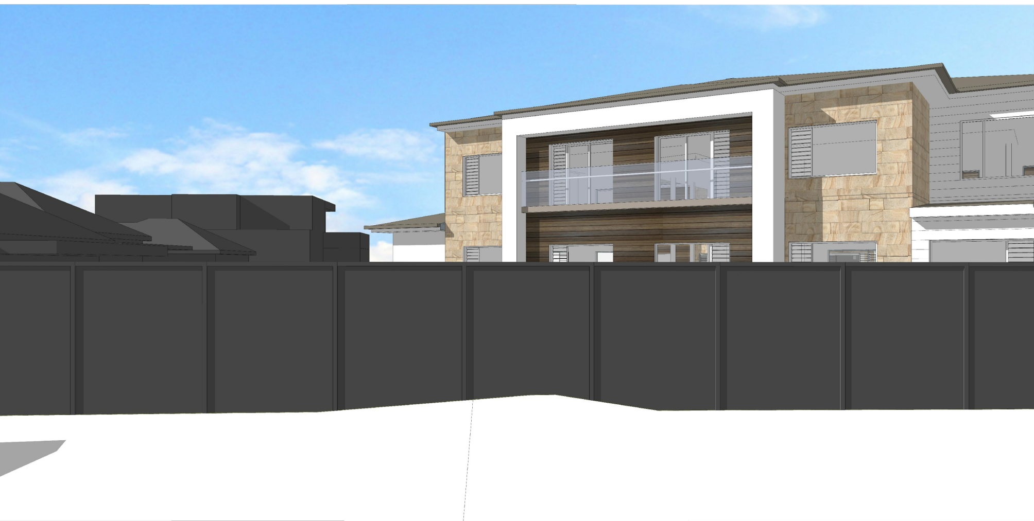
PROPOSED SCHEME, 3 STOREY Ground Floor - 6m Setback First Floor - 6m Setback Second Floor - 6m Setback - NOT VISIBLE
